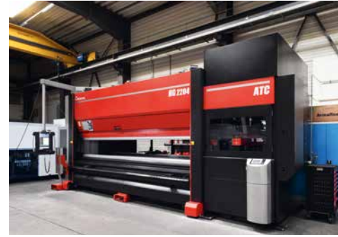
Kraftpaket: Amada HG2204-ATC Biegepresse
